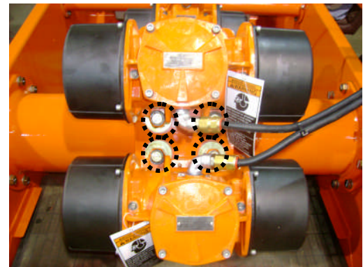
Figure 25 Motor Bolts – Four Per Motor
