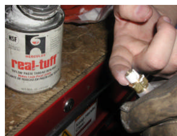
Figure 16 Sealant Used on Plug Threads
