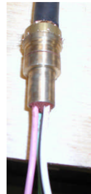
Figure 38 Compound Tube Filled with Epoxy Compound
