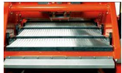
Figure 20 Screens & Wedges Firmly In Place
