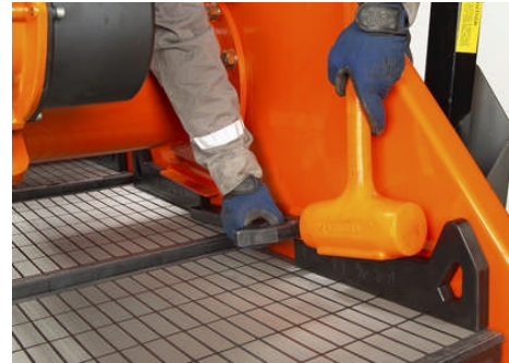
Figure 21 Meerkat Screen Removal
