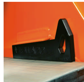
Figure 23 Wedge Positioned Between Screen Surface & Support Bar
